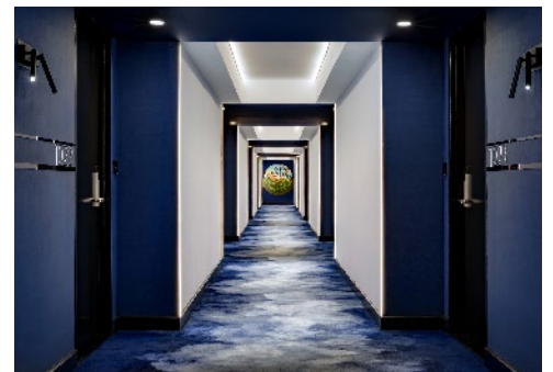
▲ Cove lighting helps illuminate hotel corridors.
