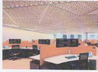
Signature Ceiling Approximately 4,000 modular, bespoke ceiling panels combine 2.5 million metal 'petals' with half a million LED lights.
